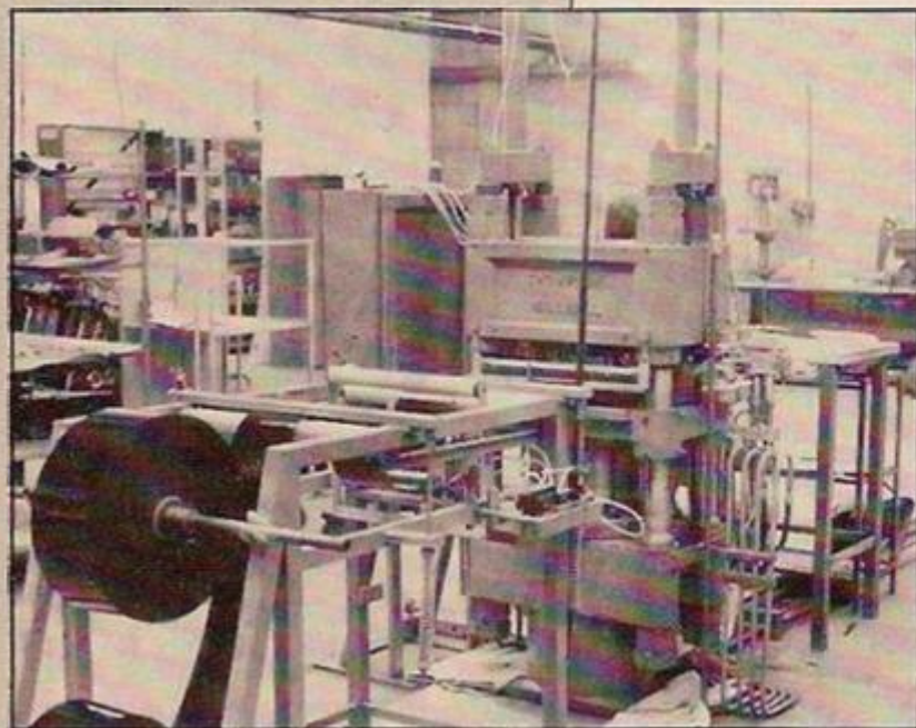
A roll of black vinyl feeds into the press to be stamped with the program cut into squares and stacked.
